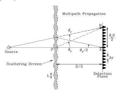
Figure 11.7 Scattering screen and multipath propagation.
