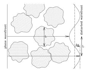
Figure 11.6 Refractive distortion of an electromagnetic wave propagating through the ISM with electron density variations on a length scale  $\sim L$ . The characteristic scattering angle is  $\theta \approx \Delta x/L$  (see text).
